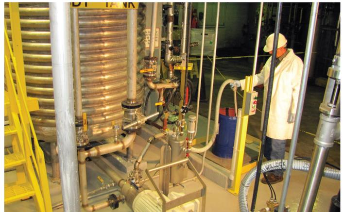
The dye container rests on a scale alongside the mixer, and the mix proportions are monitored closely to guarantee the accuracy of the final solution.
