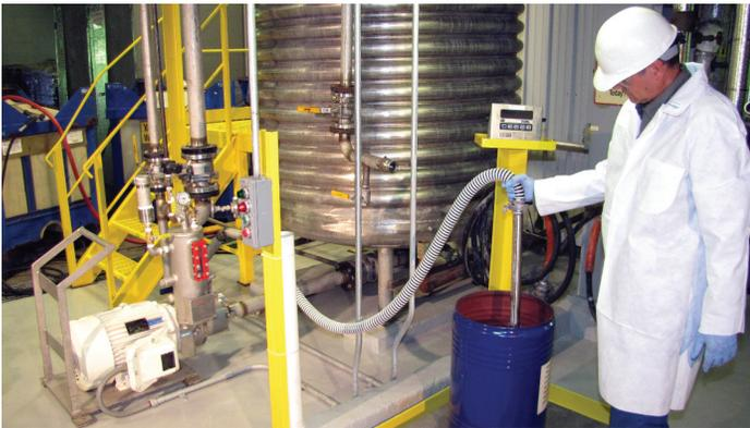
The dye container rests on a scale, which enables the operator to monitor powder injection and prepare an accurate solution. The injection cycle in this application typically requires about eight minutes.
